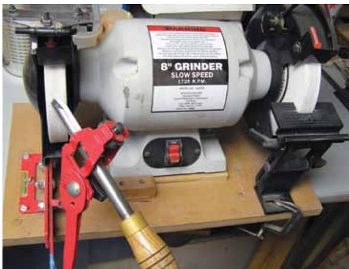
For everyday sharpening, many woodturners rely on a slow-speed grinder with two 8" x 1" white aluminum oxide wheels. On Jim Echter's machine, the left wheel has a TruGrind jig for sharpening gouges, skewers, and parting tools. The right has a Veritas adjustable-angle platform for sharpening scrapers.
