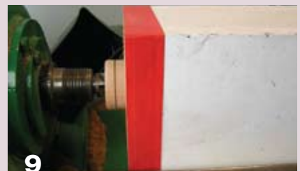
7 The shoulder is finished and it's time to turn the tenon.
