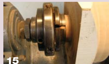
15 Remount the tenon of the newel post cap into a 4-jaw chuck using the turned groove as a marker for the teeth of the chuck.
