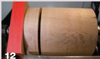
12 Layout lines are marked and the first key dimension is created using a parting tool.
