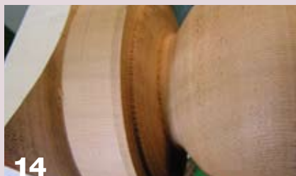
14 The cap is rough turned and ready for decorative beads and sanding.
