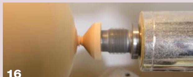
16 Cut away the tenon from the top part of the newel post and sand that area.
